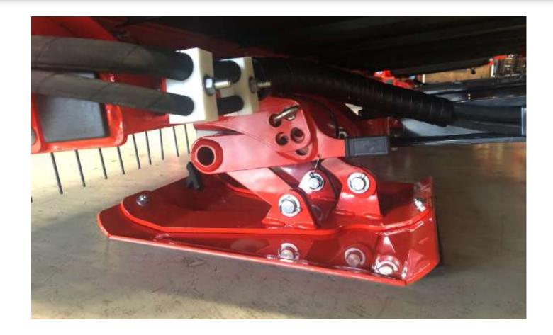
✓ On the MM 760, the raking height is adjustable by changing the position of a pin
